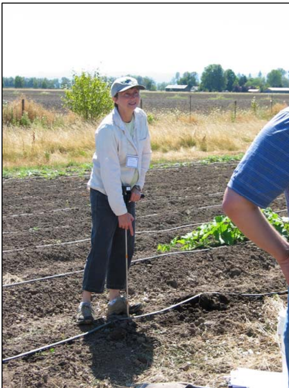
Teresa demonstrates the use of a soil penetrometer to determine surface and subsurface compaction at Fairfield Farm during the August 2010 Soil Quality Project Workshop field tour.
