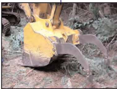
Bucket of excavator with attached shanks and wings.
